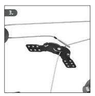
3. Open the lockout device by rotating the locking lever to the left. Place the device over the cable loop, holding the cable in its tightest position.
