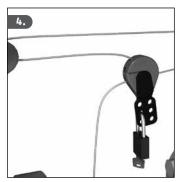
4. Placement of the lock shackle into any one of the six holes will prevent the locking lever from being opened.
