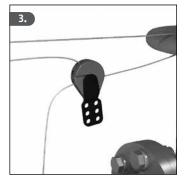
3. Rotate the black locking lever back to the right and into the locked position. Pull the cable to the desired length. The cable cannot be removed from the locking device once the black lever is in this position.
