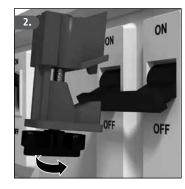
Turn the adjustment wheel of the lock counterclockwise to open the lockout device as far as necessary.
