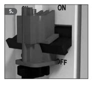
5. If the device sits tightly and securely on the connection bridge of the circuit braeaker and prevents the "On" position from being set, turn the screw wheel clockwise until the openings in the screw wheel coincide exactly with the through holes in the lock.
