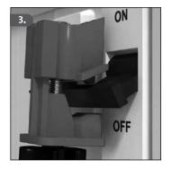
Position the circuit breaker lockout device on the circuit breaker so the tongue of the lock engages in one of the spaces between the individual circuit breaker rockers behind the connection bridge.
