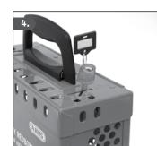
2. Safely isolate the individual power sources and collect the appropriate keys inside the SAFETY REDBOX™.
